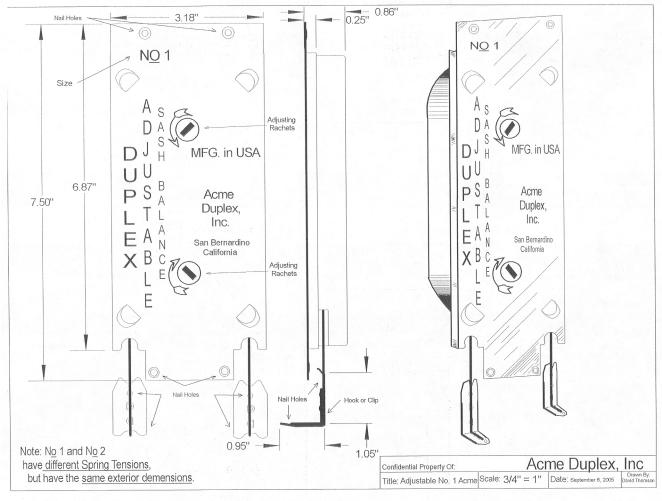
**DUPLEX®** balances require no special framing for overhead balance space, nor stud mortises at sides. Balances are installed approximately midway between sill and head jamb and 2" above center, and fit virtually in the pulley stile thickness. (Two cables per balance.)
